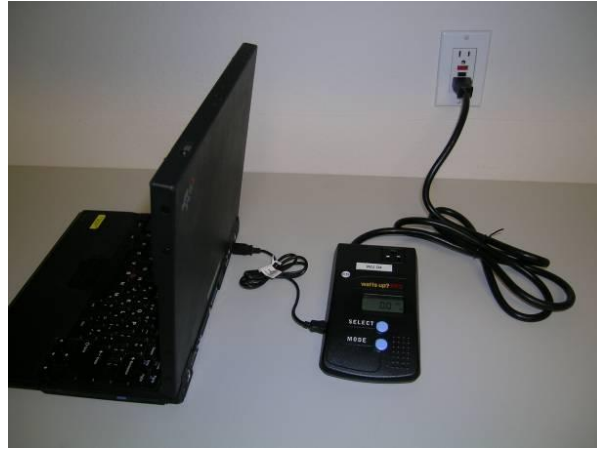
Figure 4. Meter Connected to Computer for Downloading Data
